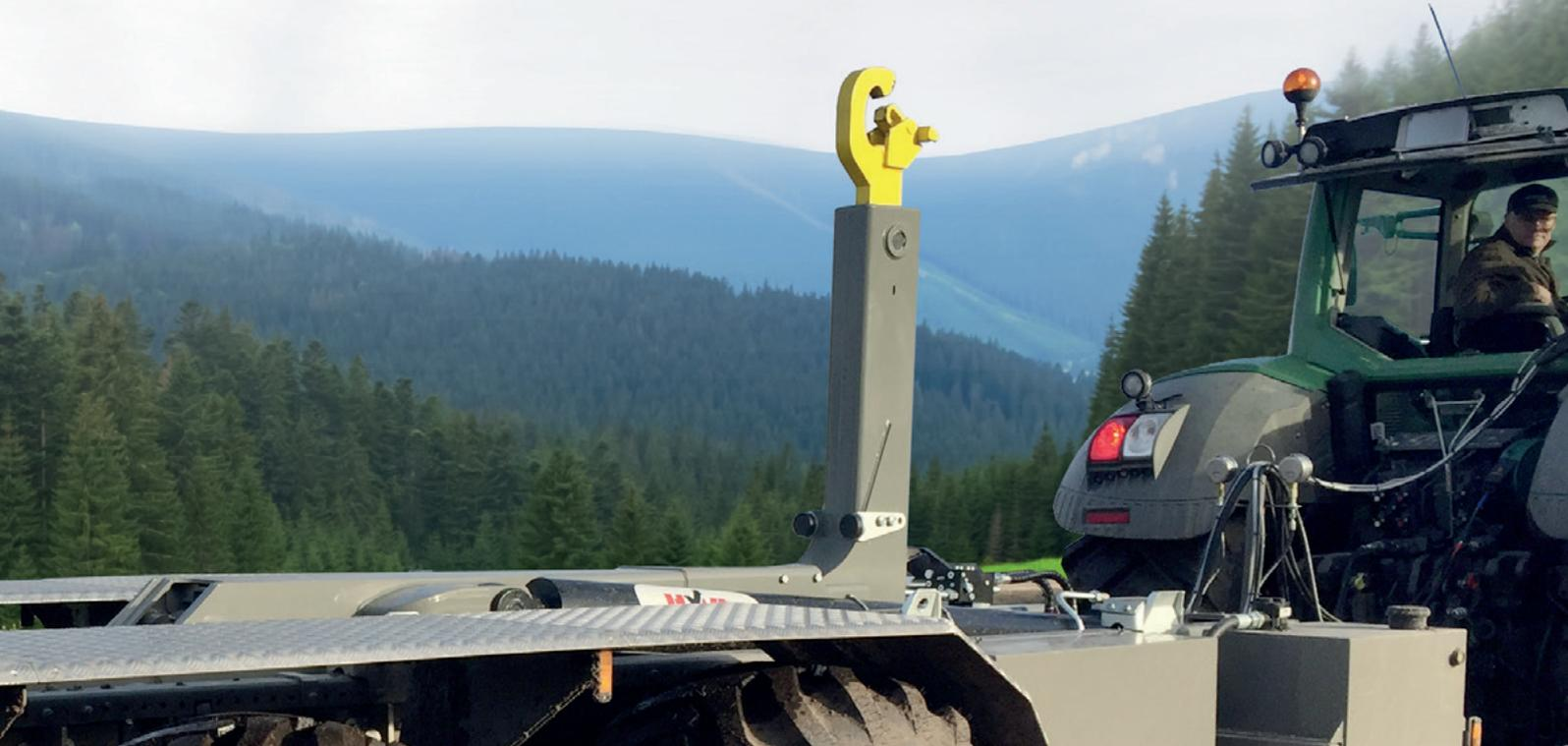
A fully automatic hydraulic drive system, the Copro-Drive System integrates tractor and machine drive systems into a single road train unit that copes with difficult terrain.
